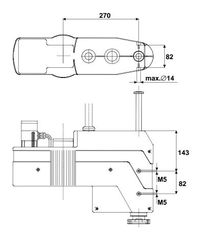
Make sure that the entire load capacity of the robot with all of its attachments, grippers, and workpieces does not exceed 5 or 8 kg.
