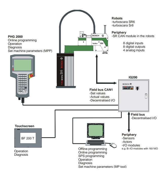
The robot system SR6/SR8 consists of robust robotic mechanics with four freely programmable axes. With its high velocity and high loading capacity (up to 8 kg) the robot is predestined for assembly work and for fast Pick & Place motions.
