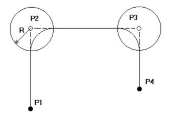
In practice, the driving time of the third axis is usually responsible for how much driving time is saved. In this case the following can be generalised: depending on lift and defined passing area, a saving of up to 50% of the drive time of the third axis can be achieved. When determining the passing area, existing interferences (edges of pallets, boxes, crates) in the path must be taken into account!
