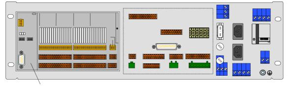
B~IO Module (not included in the standard scope of delivery)
