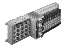
The VTS02 valve block system is a flexible modular system for achieving your pneumatic tasks. 3/2, 5/2 and 5/3 directional control valves can be combined at will on a maximum of 16 valve positions. The electrical controlling occurs via field bus system. With the CAN bus module, the VTS02 can be configured for the rho4.1 and can be hooked up to the IQ200.
