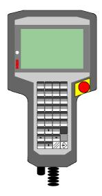
BAPS3 programs can be constructed and tested directly on the controller with the PHG2000. Furthermore, data from an application program can be displayed or inquired. The following operational functions can also be carried out:
