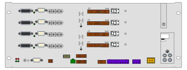
The power supply for the logic voltage of the drive unit is gained from the IQ200 power supply unit. The provision of the required intermediate circuit voltage for the power stage occurs via the servo power supply, which is standardly supplied in single-phase via the X50 interface
