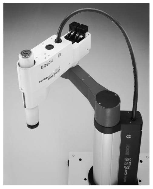
**turbo***scara* **SR6/SR8 dust proof** is for use in especially severe conditions. This robot is completely sealed and uses the full scope of the turboscara family performance characteristics in dusty or wet work areas.
