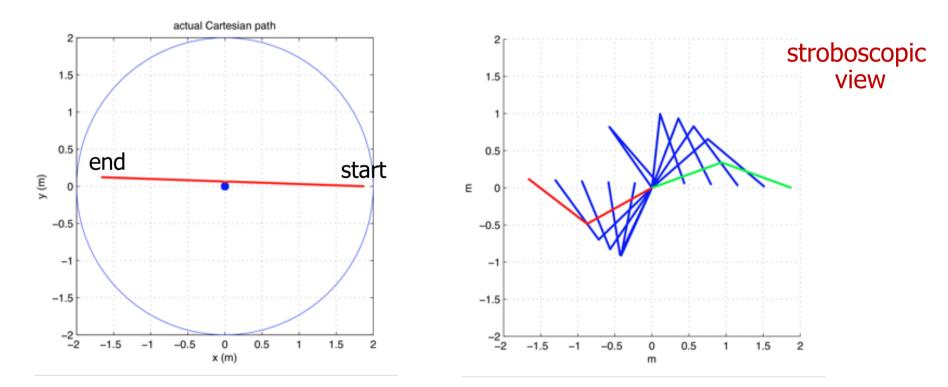
a line from right to left, at  $\alpha = 178^{\circ}$  angle with *x*-axis, executed at constant speed v = 0.6 m/s for T = 6 s
