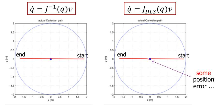
a line from right to left, at  $\alpha = 179.5^{\circ}$  angle with *x*-axis, executed at constant speed v = 0.6 m/s for T = 6 s
