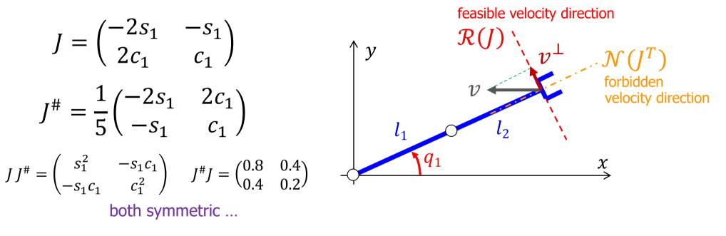
$\dot{q} = J^{\#}v$  is the minimum norm joint velocity vector that realizes exactly  $v^{\perp}$ • at  $q_1 = \pi/6$ : for  $v = \begin{pmatrix} -0.5 \\ 0 \end{pmatrix}$  [m/s],  $\dot{q} = J^{\#}v = \begin{pmatrix} 0.1 \\ 0.05 \end{pmatrix}$  [rad/s]  $\Rightarrow v^{\perp} = JJ^{\#}v = \begin{pmatrix} -1/8 \\ \sqrt{3}/8 \end{pmatrix}$  [m/s]
