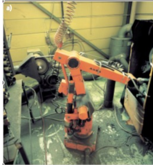
ASEA IRB-6 (1973) first robot all-electric-drives
