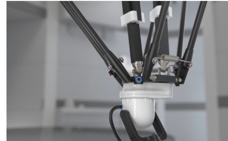
ABB 365 Flexpicker 5-DOF Delta parallel kinematics
