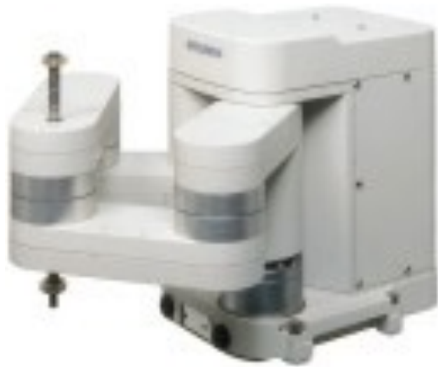
Mitsubishi RP (repeatability 5 micron, payload 5 kg)
