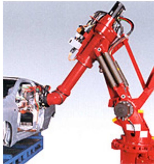
Comau Smart H4 closed kinematic chain
