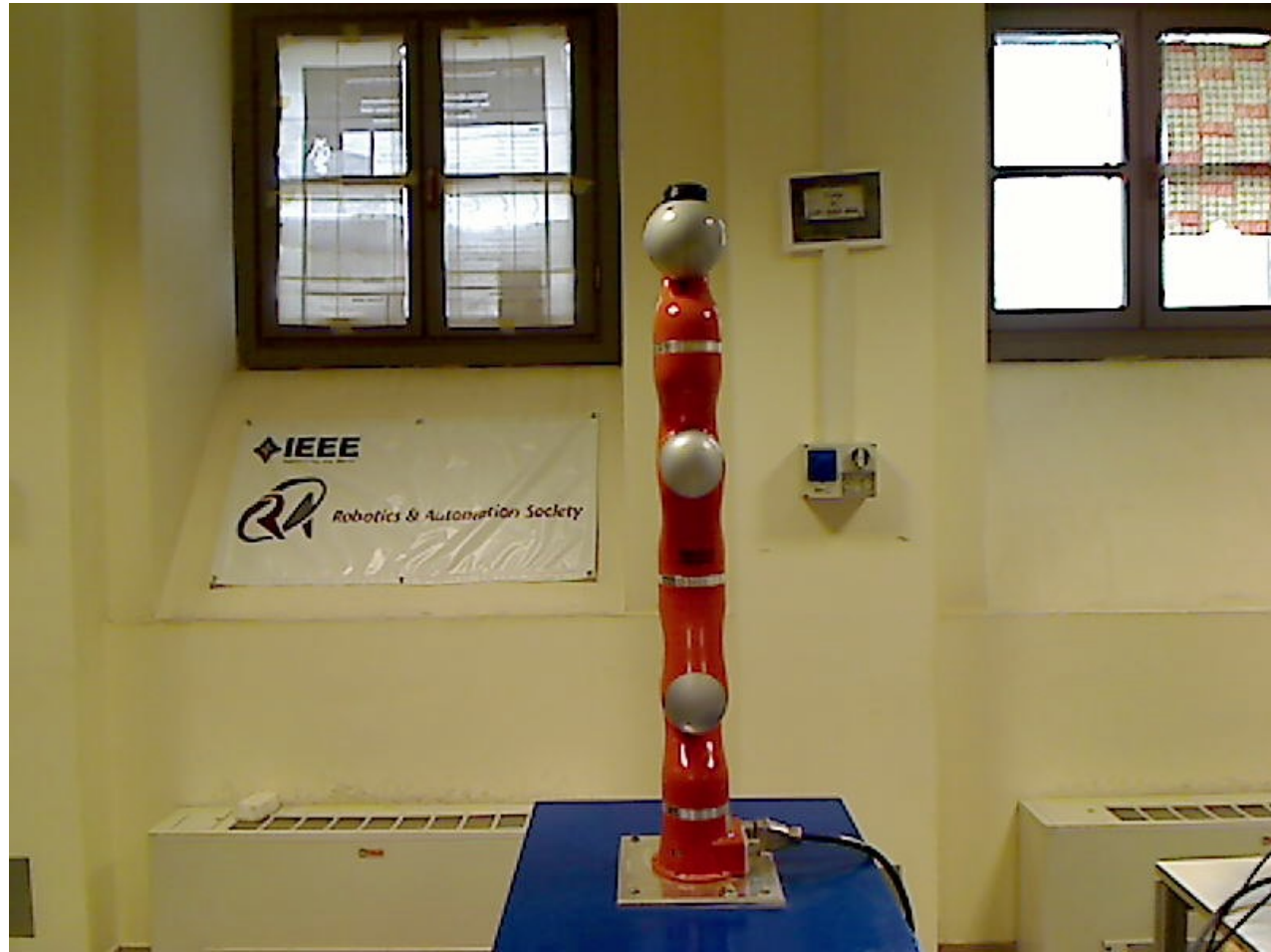
KUKA LWR4+ (lightweight, about 14 kg)
