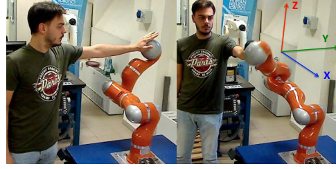
Fig. 7. The set-up and the Cartesian reference frame for the contact force control experiments. On the left, the human is pushing along the Y direction where a non-zero desired force is specified ( F_{y,d} = 15 N). On the right, a drift effect occurs due the absence of a human reaction in the Y direction (a force is applied approximately along the X direction only).
