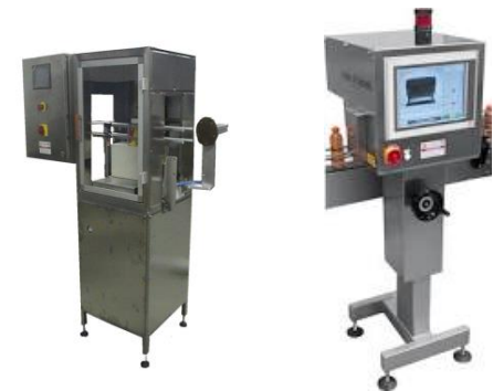
Level-Cap-Printed Code Inspection
