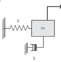
• This system was shown to be passive w.r.t. the pair (u, y) with u = f,  $y = \dot{x}$ , and as storage function the total energy (kinetic + potential)
