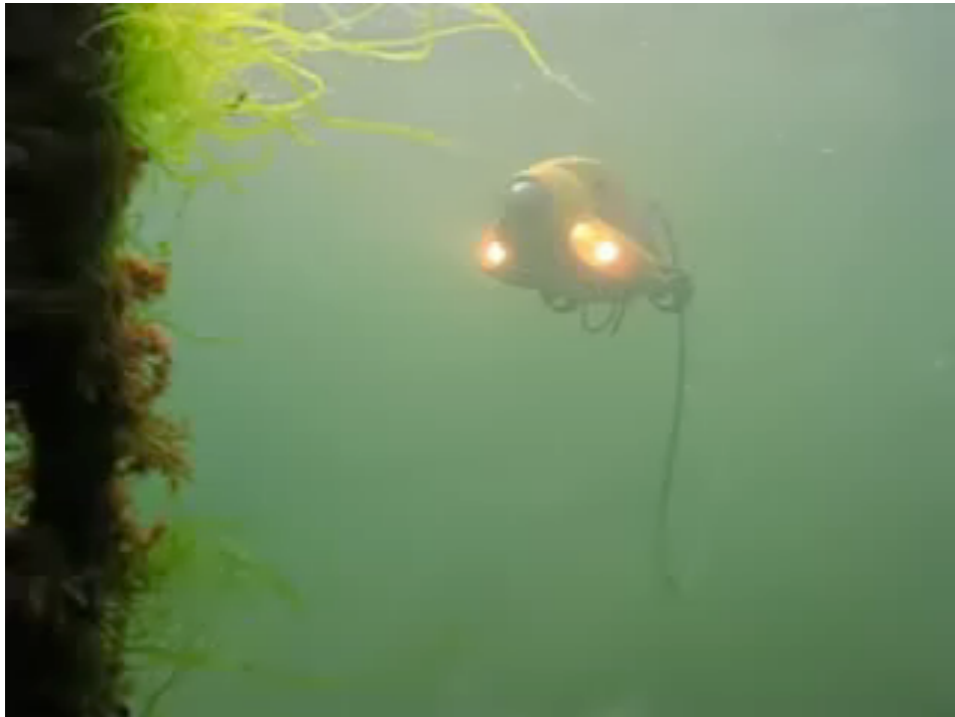
Seagoo ROV (inspection)
