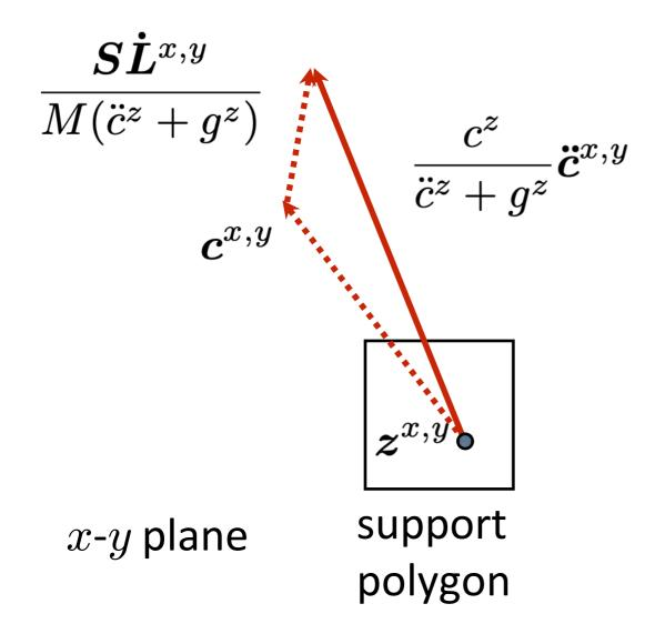
aside from the effect of internal angular momentum variations, the CoM horizontal acceleration is the result of a **force pushing the CoM away** from the CoP
