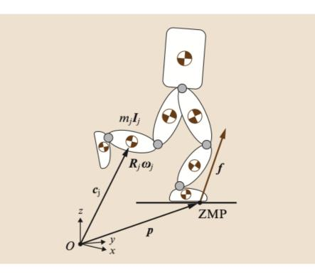
•  $\hat{q}$  is the vector of joint angles: if the floating base is fixed, a humanoid robot is exactly described like a manipulator
