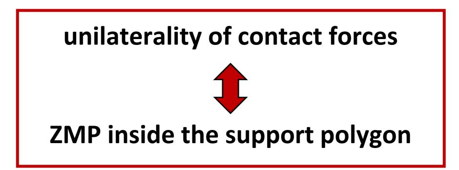
this can be interpreted as a non-tilting condition, that will ensure that the foot is well planted on the ground
