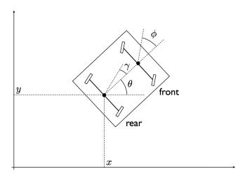
Both two-wheel axles can be assimilated to a single wheel located at the axle midpoint. The equivalent robot has then two wheels: the front wheel, which can be steered, and the rear wheel, which can be steered and driven. The k=2 kinematic constraints acting on the robot are therefore (one pure rolling condition for each wheel):
