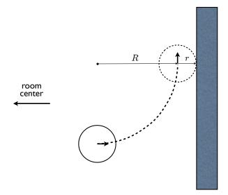
Consider the initial arrangement shown in figure. Clearly, the only way for the unicycle to avoid collision with the wall is to turn left (or right) as much as possible, by choosing  $\omega = \bar{\omega} \ (\omega = -\bar{\omega})$  for as many consecutive intervals as needed. This obviously corresponds to the robot moving along an arc of circle of radius  $R = \bar{\nu}/\bar{\omega}$ . The desired clearance is therefore  $r + R = r + \bar{\nu}/\bar{\omega}$ .
