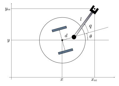
Refer to the figure for the definition of the relevant variables. The configuration vector of the mobile manipulator is  $\boldsymbol{q} = (x \ y \ \theta \ q)^T$ . The corresponding kinematic model is
