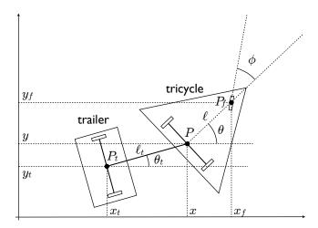
The kinematic constraints acting on the robot are therefore three (one "pure rolling" condition for each wheel):
