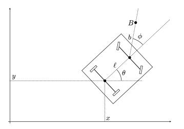
to put the equations of the bicycle in the input-output linearized form:
