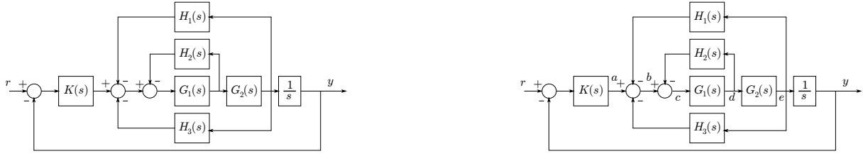
Figure 3: Ex. 5 – The automatic steering control scheme (Left) and the chosen signals (Right)
