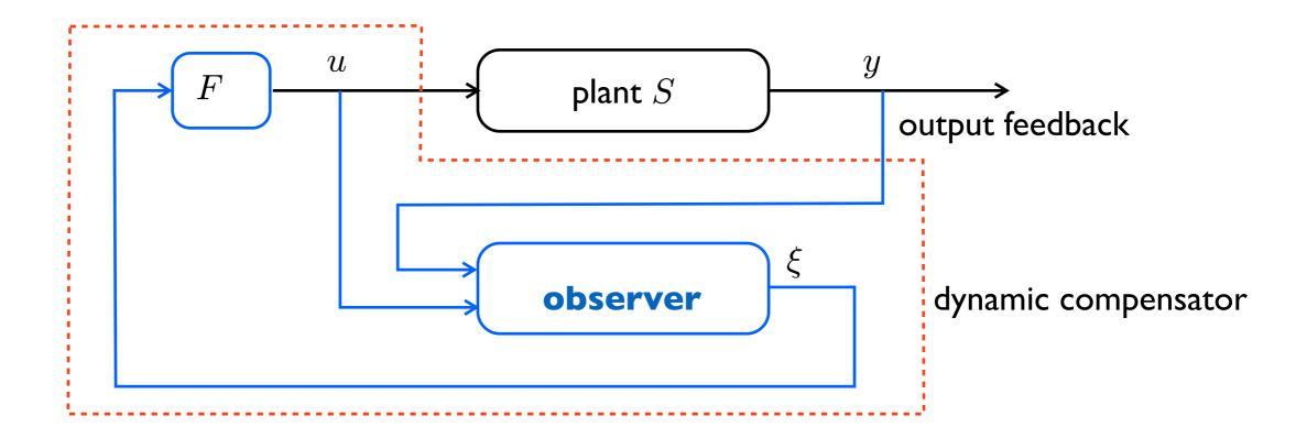
if we rewrite the asymptotic observer system as  $\xi=(A+BF-KC)\xi+Ky$  and note that the output of the dynamic compensator is  $u=F\,\xi$  we can compute the transfer function from y to u of the controller (dynamic compensator) as
