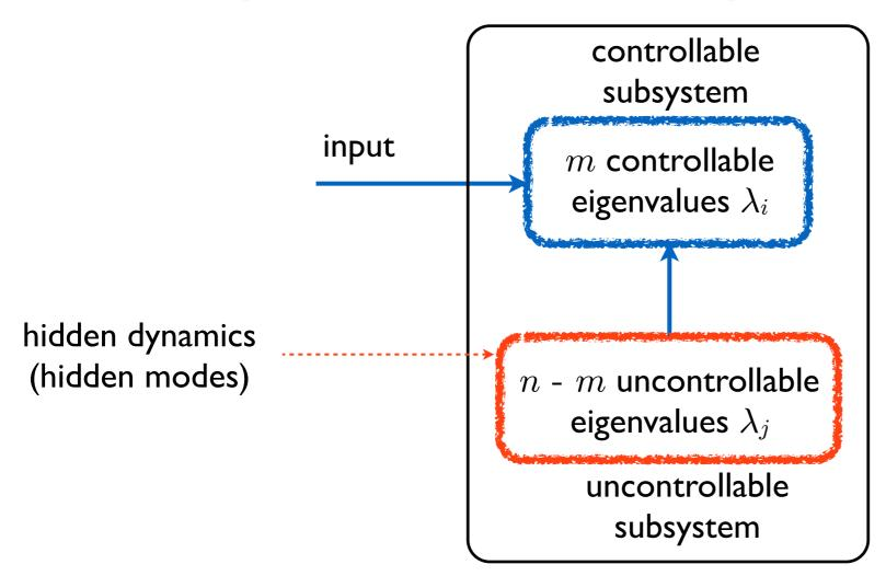
effect of a state feedback (system is no more fully controllable so the previous result on eigenvalue assignment is not applicable)
