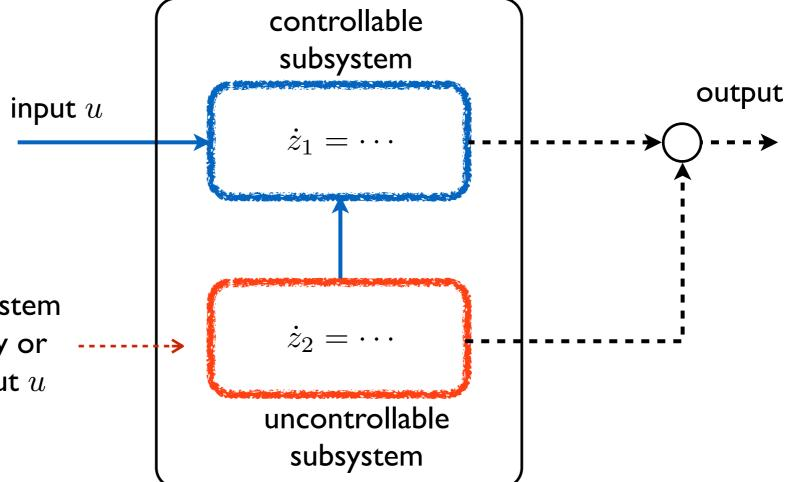
the state evolution of this subsystem indirectly through  $z_1$ , by the input u
