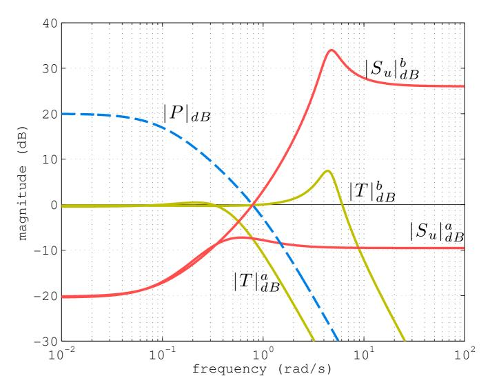
closed-loop bandwidth increase from  $B_3{}^a$  to  $B_3{}^b$
