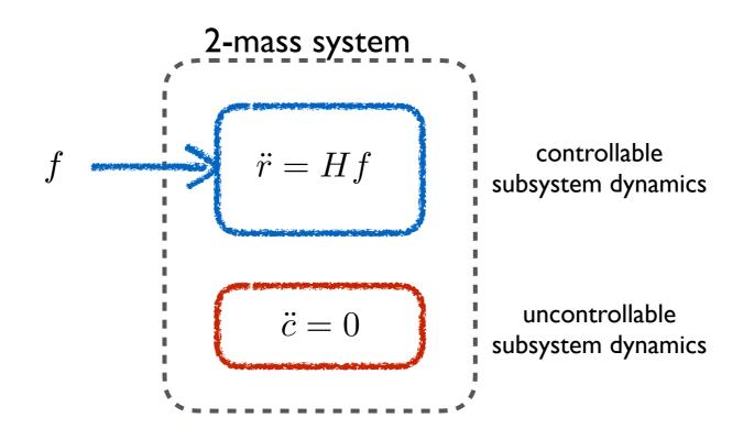
The Kalman decomposition, starting from these new coordinates, highlights similar controllable and uncontrollable subsystems (the new coordinates are practically a rearrangement of the old ones)
