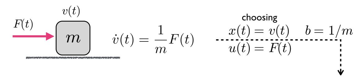
$$\dot{x}(t) = 0 \cdot x(t) + b \cdot u(t) \quad \text{and} \quad \text{same} \quad \dot{x}(t) = b \cdot u(t)$$
