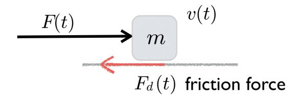
we add a viscous friction force  $F_d(t)$ , acting on the mass, which can be considered proportional to the velocity (this is a modeling hypothesis) and acts in the opposite direction w.r.t. the motion, that is  $F_d(t) = \mu \ v(t)$  and with  $\mu > 0$
