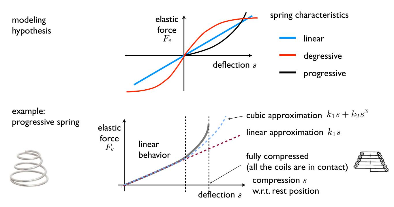
the (linear) approximation of the spring characteristic is part of the modeling phase similarly for the hypothesis on the friction force
