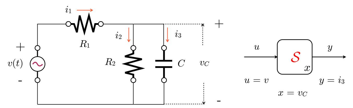
one energy storage component and therefore the state is a scalar (here  $x=v_C$ )
