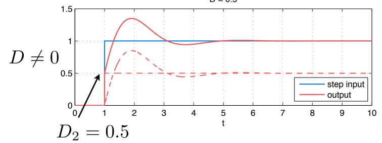
at time t = 1, the input switches from 0 to 1 and instantaneously the output switches from 0 to  $D_2 u(1) = D_2$
