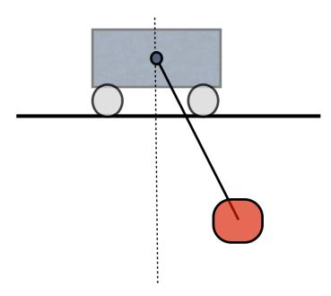
crane control: how control can help an inexpert operator who has to move a payload with a crane - here using a technique called "input shaping" (Georgia Tech)
