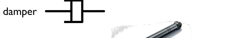
a mechanical damper is also called dashpot
