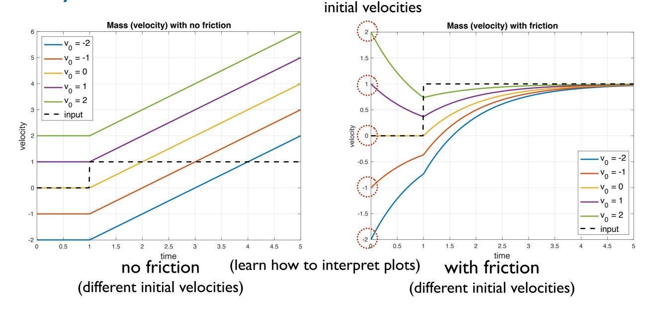
velocity time evolution when a constant 1 N force is applied from t=1 sec
