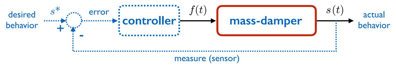
f(t) is a force (produced by an actuator)
