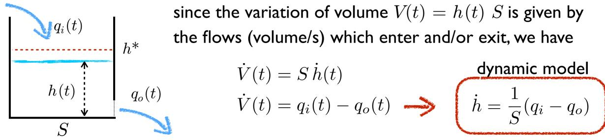
since the variation of volume V(t) = h(t) S is given by  $h^*$  the flows (volume/s) which enter and/or exit, we have dynamic mod
