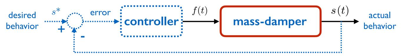
we assume that the controller produces a force f(t) proportional to the error (desired behavior – actual behavior) that is  $f(t)=k_p\ (s^*-s(t))$  with  $s^*$  constant
