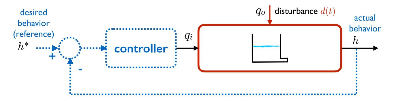
may be  $q_i$  is not the real input, but the output of a valve commanded by a voltage v: we may need to include the actuator dynamics
