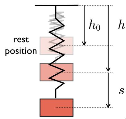
Mass-Spring-Damper model under gravity
