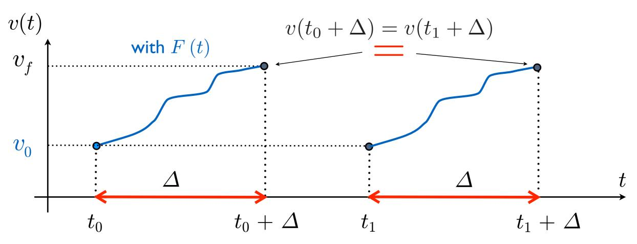
starting from the same initial condition  $v_0$  and applying the same input (force) F(t) after same time interval  $\Delta$  leads to the same state
