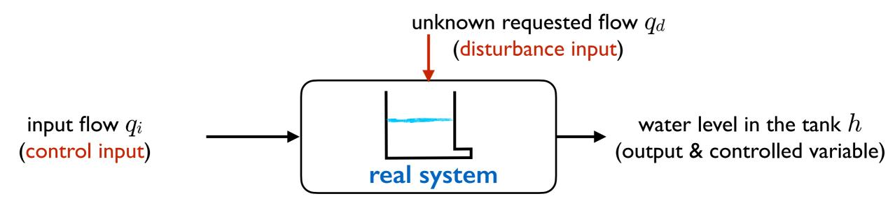
problem: we want to maintain the water level at a desired height regardless of the unknown output flow and any other disturbance (evaporation, loss in the tank,...)
