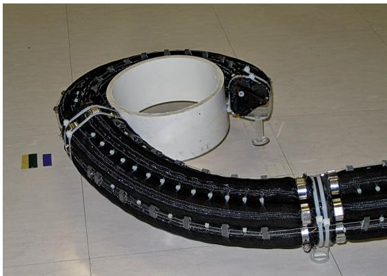
**Fig. 11.7** The OctArm continuum manipulator (courtesy I. Walker)
