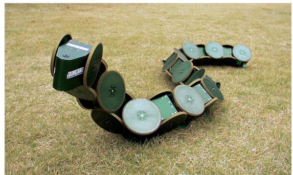
**Fig. 11.6** Active cord mechanism (courtesy S. Hirose)
