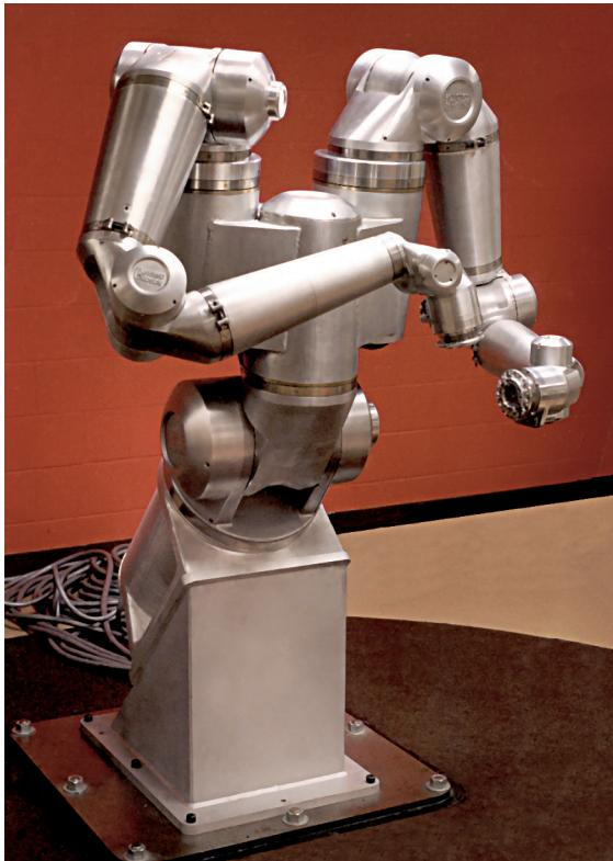
**Fig. 11.4** 17-DOF robot (courtesy Robotics Research Corporation)
