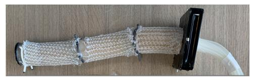
Figure 1: A pneumatic soft robot consisting of three segments. Each segment can bend in any direction by inflating its four air chambers. **Results and discussion**
