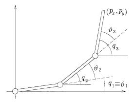
Fig. 3. A 3R planar robot with absolute and relative coordinates.
