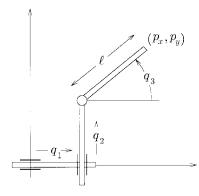
Fig. 1. A PPR planar robot.
