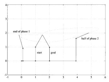
Fig. 4. Reconfiguration of the PPR robot with sinusoidal steering.
