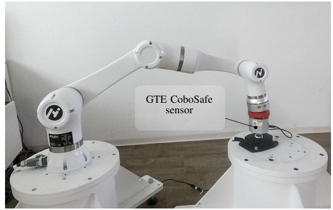
Fig. 3: Experimental setup of LARA 5 colliding with a GTE CoboSafe sensor.
