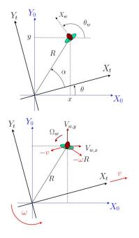
Fig. 3. Frames and variables definition: walker and platform still (top) and in motion (bottom)
