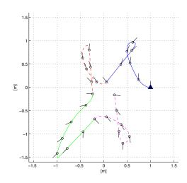
Fig. 8. Walker absolute locomotion under the platform controller (3) and (7): at start, axis  $X_t$  coincides with  $X_0$
