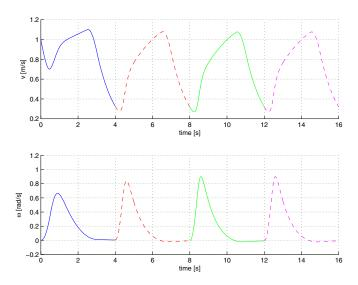
Fig. 7. Linear and angular velocity commands with controller (3-4)
