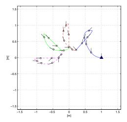
Fig. 6. Walker absolute locomotion under the platform controller (3–4): at start, axis  $X_t$  coincides with  $X_0$
