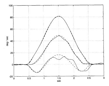
Fig. 3.4. Computed and actual velocity of joint 2 (top), joint 1 (center), and tip deformation (bottom)
