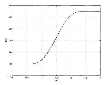
Fig. 3.1. Desired and actual trajectory for joint 1
