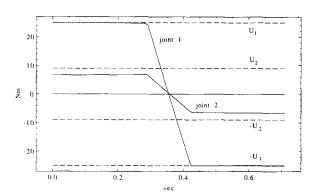
Fig. 6. Example 2. Optimal solution: torque.
