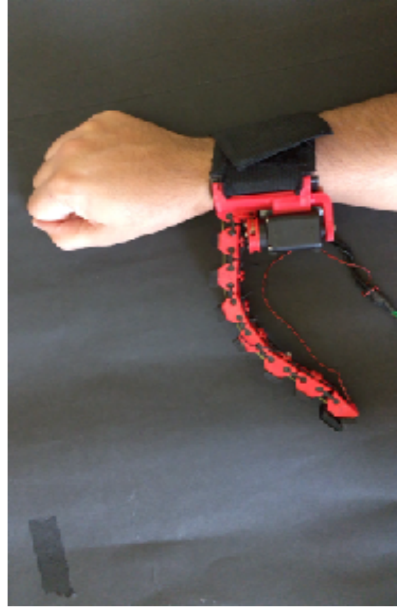
Joint compliance designed from fingertip trajectory
