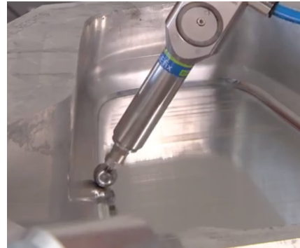
Figure 2: Robotized surface polishing of a metallic work piece.
