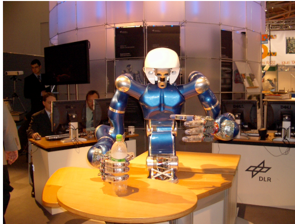
Figure 1: The DLR Justin robot, a torso with bimanual arms.
