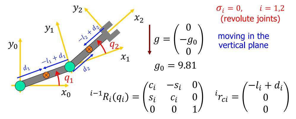
**assumption**: center of mass of each link is on its kinematic axis
