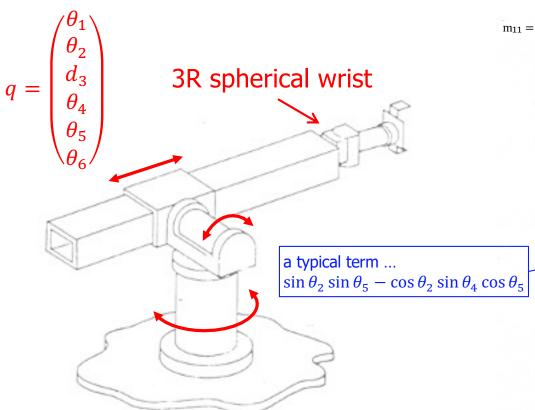
radius of gyration factors  $k_{ijj}^2$  are being used here for a body of mass  $m_i$  and moment of inertia  $I_j$  with respect to an axis  $z_j$ , the radius of gyration  $k_{ijj}$  is the distance of the mass  $m_i$  from the same axis, such that  $I_j = m_i k_{ij}^2$
