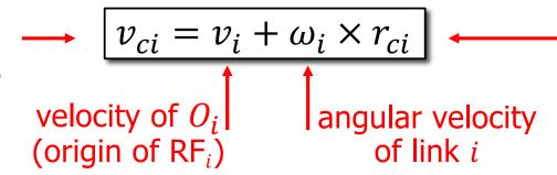
— position of center of mass of link i w.r.t.  $O_i$
