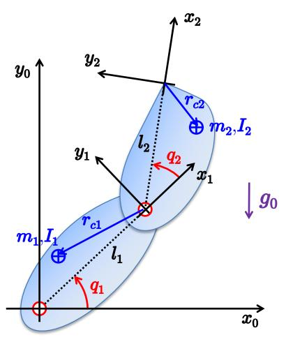
$$i^{-1}R_{i}(q_{i}) = \begin{pmatrix} c_{i} & -s_{i} & 0 \\ s_{i} & c_{i} & 0 \\ 0 & 0 & 1 \end{pmatrix}$$
