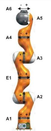
$m{Q}_{max} = (170, 120, 170, 120, 170, 120, 170)$  [deg]  $m{V}_{max} = (100, 110, 100, 130, 130, 180, 180)$  [deg/s]  $A_{max,i} = 300$  [deg/s<sup>2</sup>]  $\forall i = 1 \dots n$
