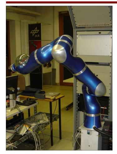
7R LWR-III lightweight manipulator: elastic joints (HD), joint torque sensing, 13.5 kg weight = payload
