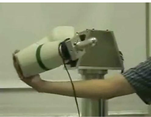
8R Dexter: self-motion with constant 6D pose of E-E (N - M = 2)
