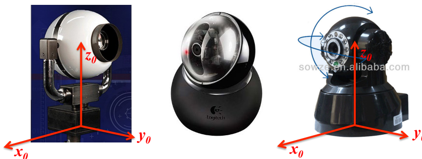
Figure 1: Pan-tilt cameras, with placement of the reference frame RF_0 (shown for two of them)
