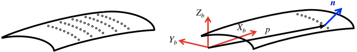
Figure 2: An aircraft plate (left) and its associated reference frame (right): The position vector  $\mathbf{p}$  locates a riveting point, where the normal to the surface is given by the unit vector  $\mathbf{n}$
