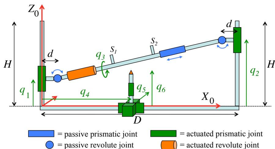
Figure 1: The 6-dof portal robot used for riveting aircraft parts (see the text for definitions and operation)
