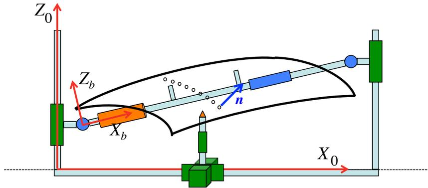
Figure 3: The aircraft plate correctly mounted on the two supports of the connecting bar of the upper section of the portal robot
