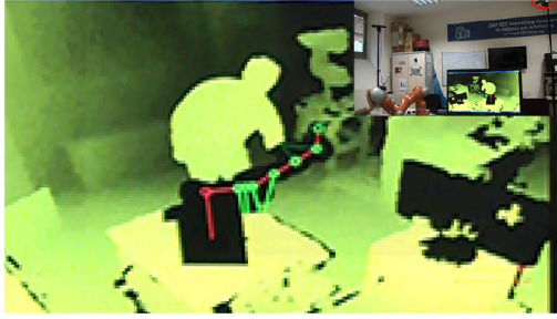
Fig. 9. In this screenshot of an experiment, the human hand is right behind the robot and thus is not detected. As a result, a collision may occur.
