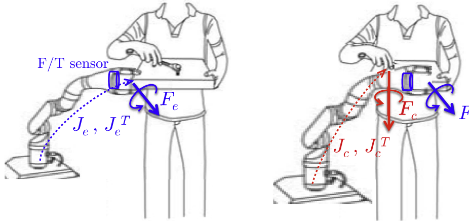
Fig. 2. Human-Robot collaboration in the presence of an F/T sensor mounted at the robot wrist. A stiff positional behavior can be achieved during manual polishing in reaction to a generalized force F_e (left), while a generalized contact force F_c can be estimated separately and in parallel, and used to reorient the robot (right).
