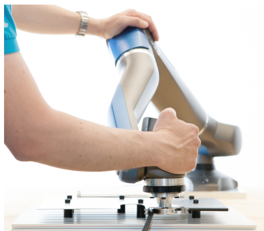
Fig. 1. Next generation of DLR lightweight robots: SARA (Safe Autonomous Robotic Assistant) in a typical collaborative task.
