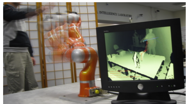
Fig. 1. A robot arm reacts instantaneously to motions of humans and other dynamic obstacles that are detected in depth space, such that collisions are avoided
