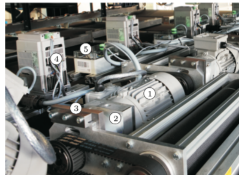
AC electric motor: 90 Nm rated torque 1.5 kW, transmission ratio 1:10
